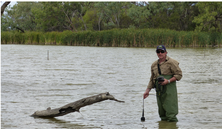
Figure 6: The Hydrolab Quanta multi-probe in Darren Ryder's (UNE) hand measures temperature, electrical conductivity, dissolved oxygen, pH and turbidity. Photo credit. Sarah Mika, UNE.
